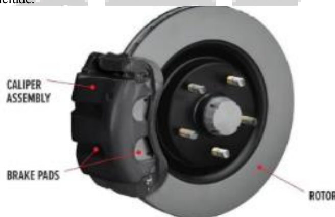
Fig. 2 – Rotors and brake pad assembly
